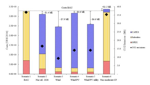
Figure 3: Comparison of all costs (primary ordinate) and CO<sub>2</sub> emissions (secondary ordinate) for each scenario. Operating costs (OPEX) include fuel costs as well as fixed and variable operation and maintenance costs. Subsidies refer to Zero Emission Credits (ZEC) for nuclear power plants. All exact values can be found in Table A.2. in the Appendix.
