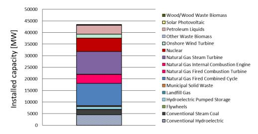
Figure 1: Technology specific installed capacity in New York [2].
